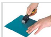
step 1: make grid cutting on surface
