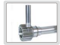
ultrasonic probe to test narrow areas (remove the cover)
